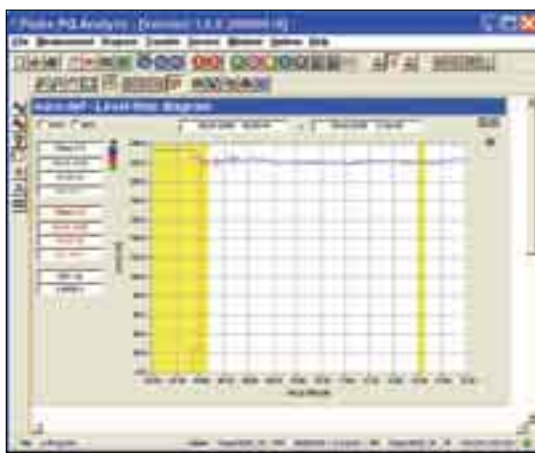
The 1760 provides flagging of data according to IEC 61000-4-30 Class-A. The flagging feature alerts the user that a dip, swell, or interruption occurred during a specific time interval. Values out of nominal ranges are marked by either a colored background or with a flag symbol.
