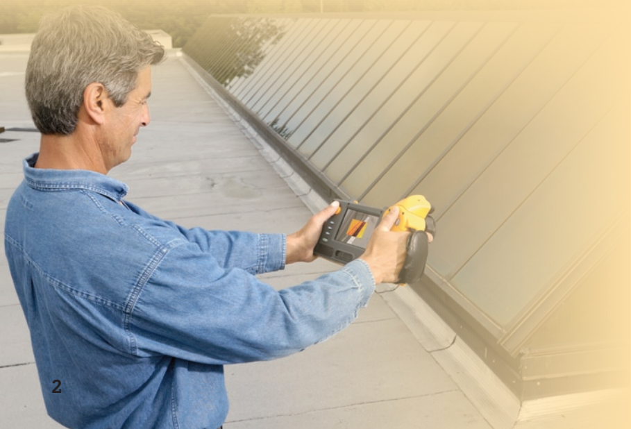
Energy audits: Perform residential and commercial energy audits by scanning for heating or cooling (energy) loss, moisture invasion, and HVAC/R problems.
